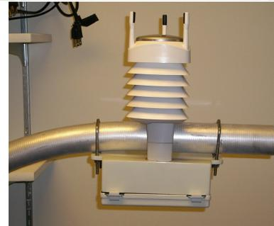
Figure 2: **Sensor Node Hardware. Top: The Soekris net4826 mounted in enclosure with power supply at left. Bottom: NEMA-6 weatherproof enclosure mounted on streetlight armature with Vaisala WXT510 Weather Sensor attached (WiFi antennas not shown).**
