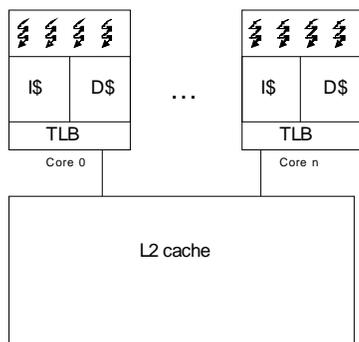
Figure 1. A schematic view of a CMT processor
