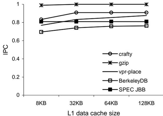
**Figure 7.** Pipeline utilization as function of cache size.
