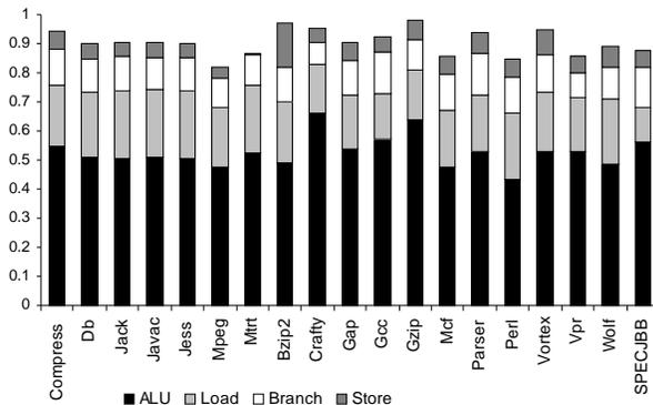
Figure 6. Fractional instruction mixes of integer workloads from SPEC JVM suite, SPEC CPU (int), and SPEC JBB.
