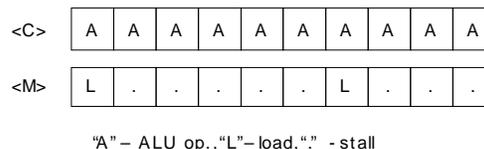
Figure 2. Compute-intensive vs. memory-intensive thread.
