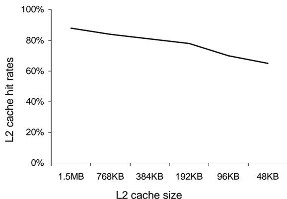
Figure 9. L2 hit rates as function of L2 size.
