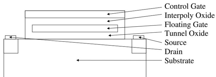
Figure 6.1: The layout of a flash cell [3].
